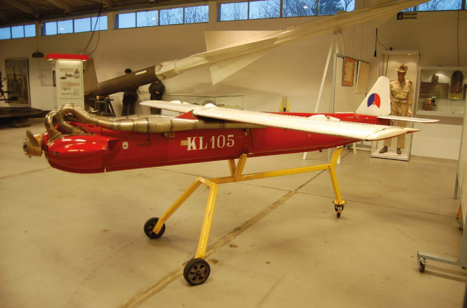
Figure 6 Northrop (Radioplane) OQ-19 Unmanned aerial target-towing aircraft for anti-aircraft artillery, used around the 1960s. Source: Historische Collectie Grondgebonden Luchtverdediging (HCGLVD), Venray, Netherlands
