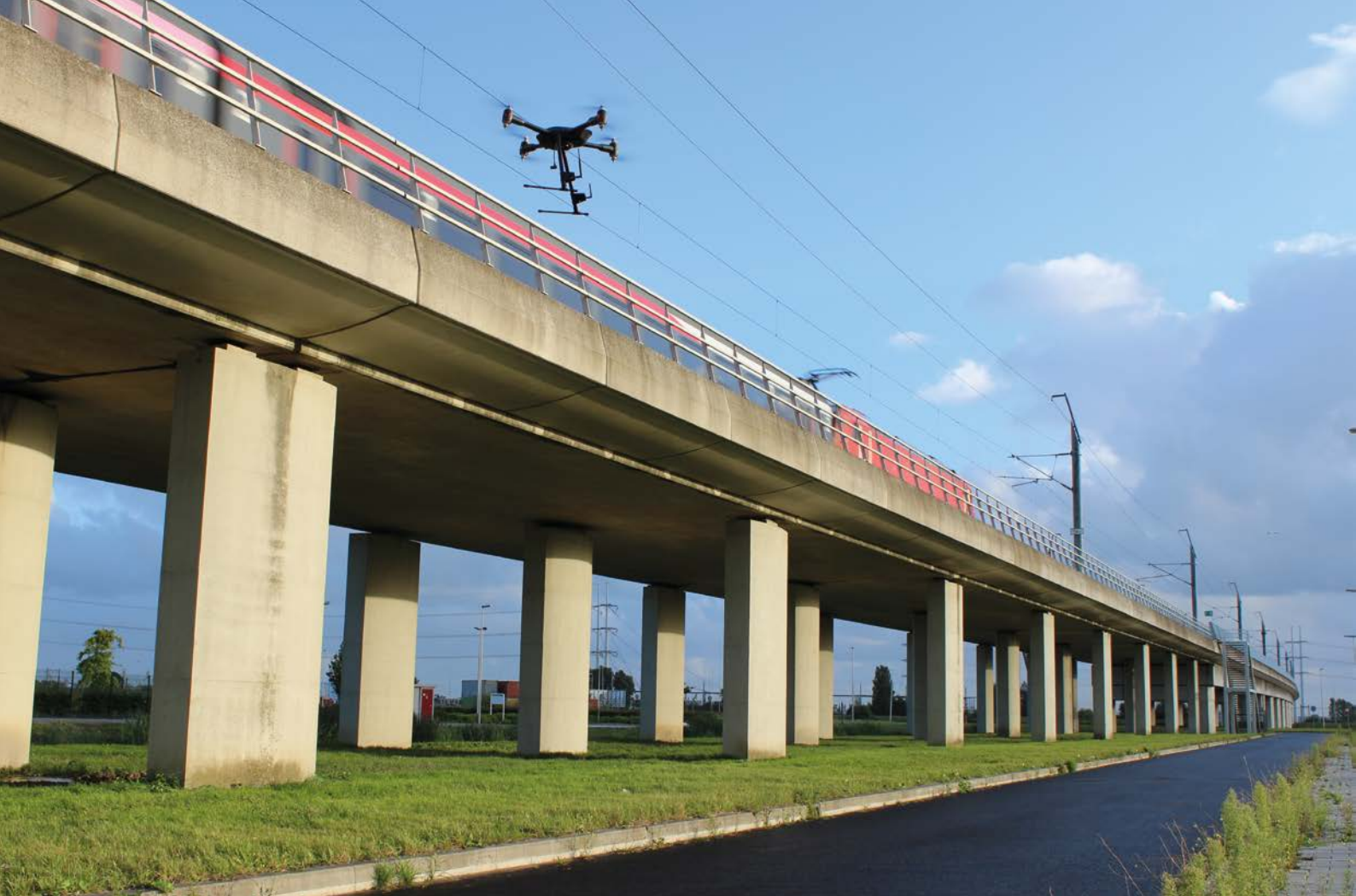
Figure 15 Use of the Zenith for security inspections of critical infrastructures Source: Aerialtronics
